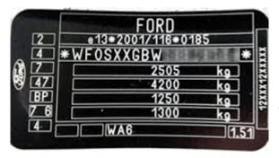
This is a typical vehicle VIN plate. It contains four weights;
